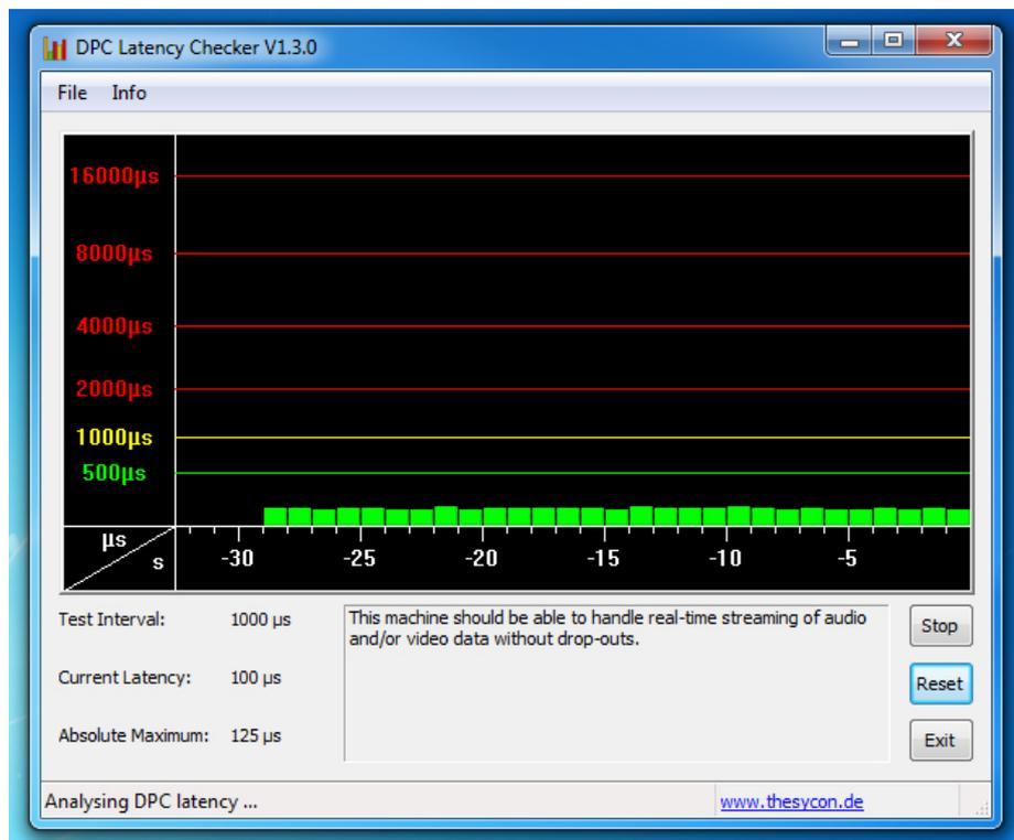
If purchasing a PC specifically for audio, or indeed video use, the Latency Checker may be copied onto a USB stick and run on machines in the computer store to check suitability.
