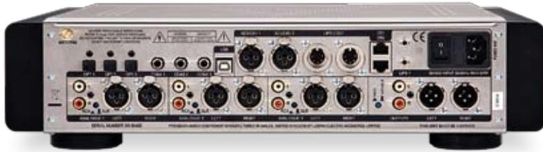
**ABOVE:** The Libra has 12 digital inputs: Bluetooth, USB, 2x AES/EBU (XLR), 2x I<sup>2</sup>S (RJ45) and six S/PDIF (3x RCA and 3x Toslink optical). It has three analogue ins on RCA and balanced XLR connections plus single-ended (RCA) and balanced XLR outputs
