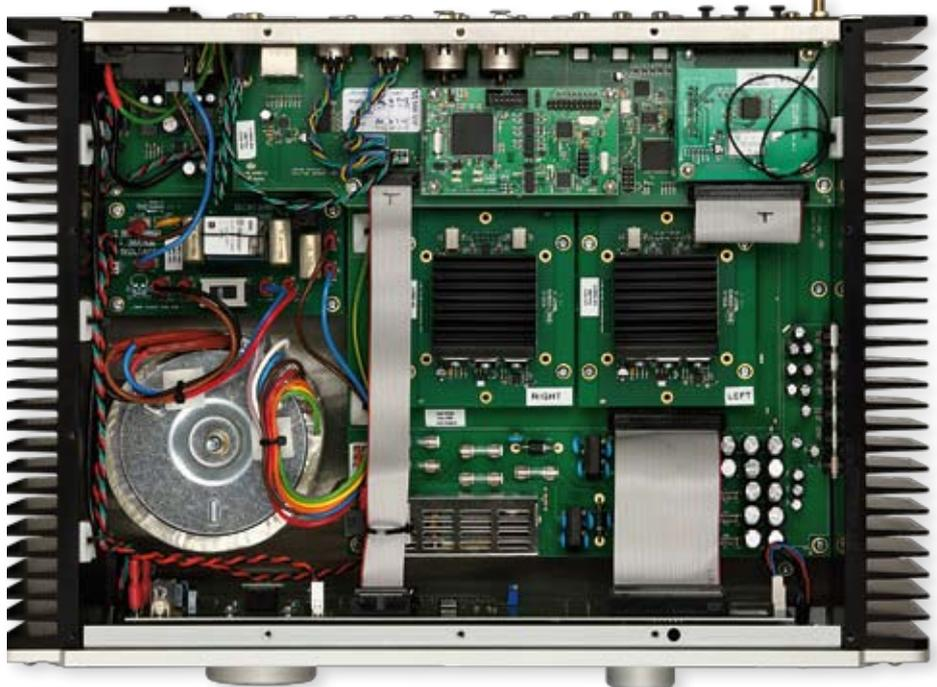
**RIGHT:** A linear PSU feeds proprietary fully balanced 'Quattro Infinity' dual-mono DAC modules [see boxout, p61] and the Thesycon driver-based 'M1' USB module. The Bluetooth can be seen top right of this picture
